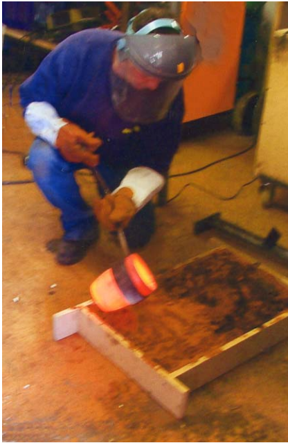
Pouring bronze into sand mould A6 crucible
