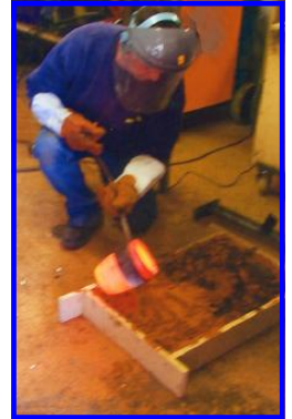
Pouring bronze into sand mould A6 crucible
