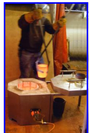
Lifting out crucible to be placed into carrying shank for casting
