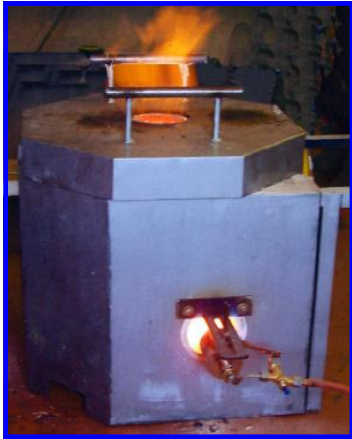
Natural draught propane fusion in action Melting Brass
